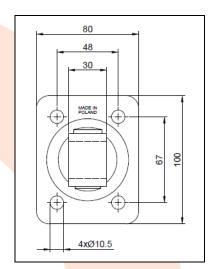
PRODUCT NAME : Adjustable hinge M20 / secured by M8 base 100x80x4
