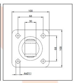
PRODUCT NAME : Adjustable hinge M20 / secured by M8 base 100x100x4
