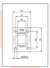
PRODUCT NAME : Adjustable hinge M16 / secured by M6 base 75x55x3
