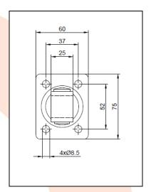
PRODUCT NAME : Adjustable hinge M16 / secured by M6 base 75x60x4
