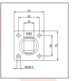
PRODUCT NAME : Adjustable hinge M16 / secured by M6 base 75x75x4
