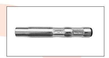
**APPLICATION**: The pipe anchor is used for embedding in solid concrete. The shape of the anchor allows it to be durable and quick seating with using much less material binding chemical anchor. The body of the anchor in the form of a cylindrical tube has a narrow diameter at the front, along which length there is an internal thread into which the hinge can be screwed. The anchor has a circumferentially
